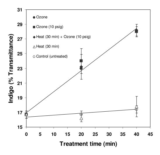
Figure A.1: Penetration of ozone across the shell of hen's eggs. Points represent the mean of measurements in experiments performed in triplicate. Error bars indicate standard deviation.
