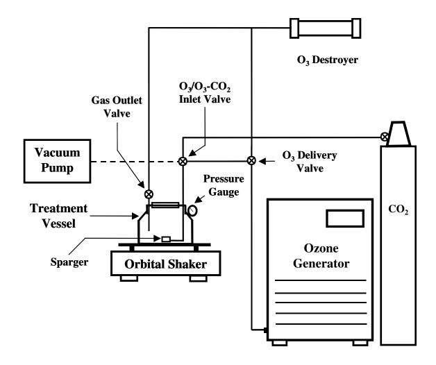
Figure 4.1: Experimental setup for treatment of shell eggs with pressurized  $O_3$  and mixes of pressurized  $O_3$  and  $CO_2$
