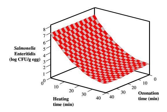
Figure 4.2: Three-dimensional representation of interaction between heating time at ambient 57°C, and ozonation time (12-14% wt/wt O<sub>3</sub>; 10 psig/69 kPa) in the elimination of *Salmonella* Enteritidis inside shell eggs. Microbial inactivation data shown were obtained from response surface model predictions (Modified from JMP IN, SAS Institute).
