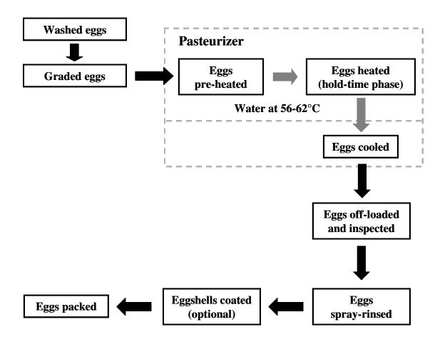
Figure 1.4: Commercial egg pasteurization (Modified from Schuman, 2000).
