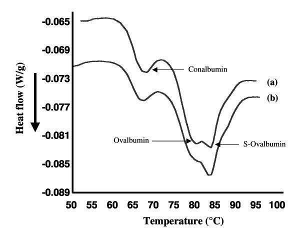
Figure 3.6: Differential scanning calorimetry thermograms of albumen obtained from (a) untreated shell eggs, and (b) shell eggs heated at ambient 59°C for 40 min. Experiments were performed in triplicate and representative thermograms are presented.
