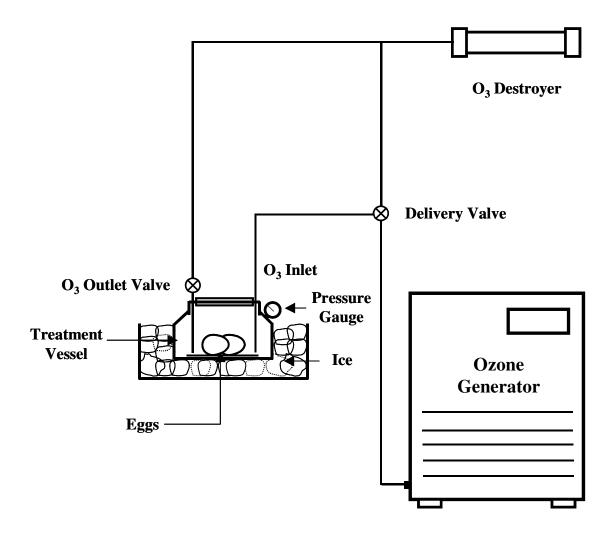
Figure 2.1: Experimental setup to treat shell eggs with gaseous ozone under pressure at low ambient temperature.
