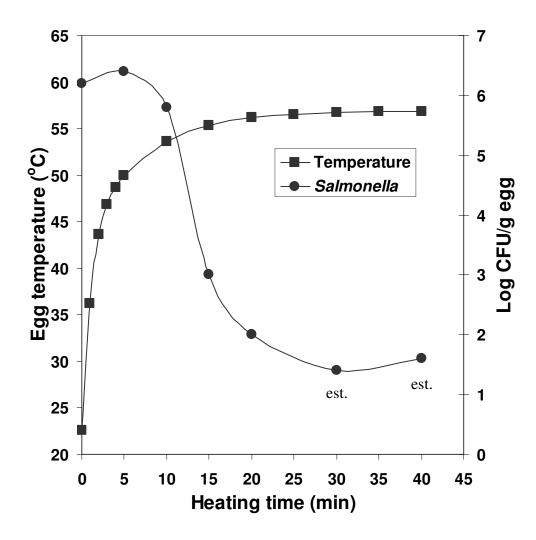
Figure 3.2: Inactivation of *Salmonella* Enteritidis in shell eggs by heat in a water bath at ambient 57°C, and increase of temperature inside shell eggs during treatment. *Salmonella* inactivation points represent the mean of microbial counts in experiments with five repeats. Points representing temperature were obtained in triplicate measurements. Estimated counts (est.) were obtained from enumeration on plates with detection limit of 10 CFU/g egg contents.
