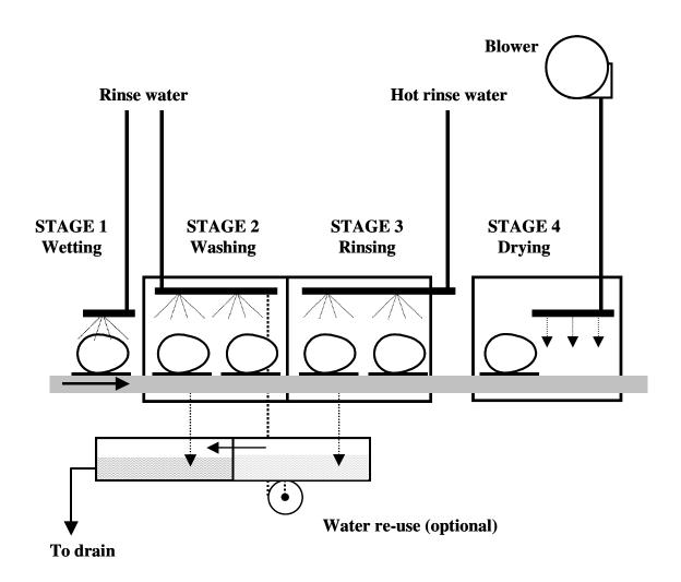
Figure 1.3: Stages of commercial egg washing (modified from Hutchison et al., 2003).
